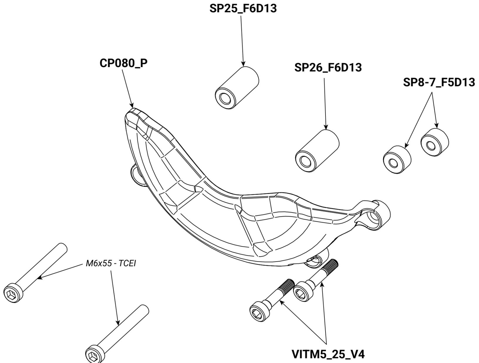
use these parts if you remove the original cable gland and captive screws
