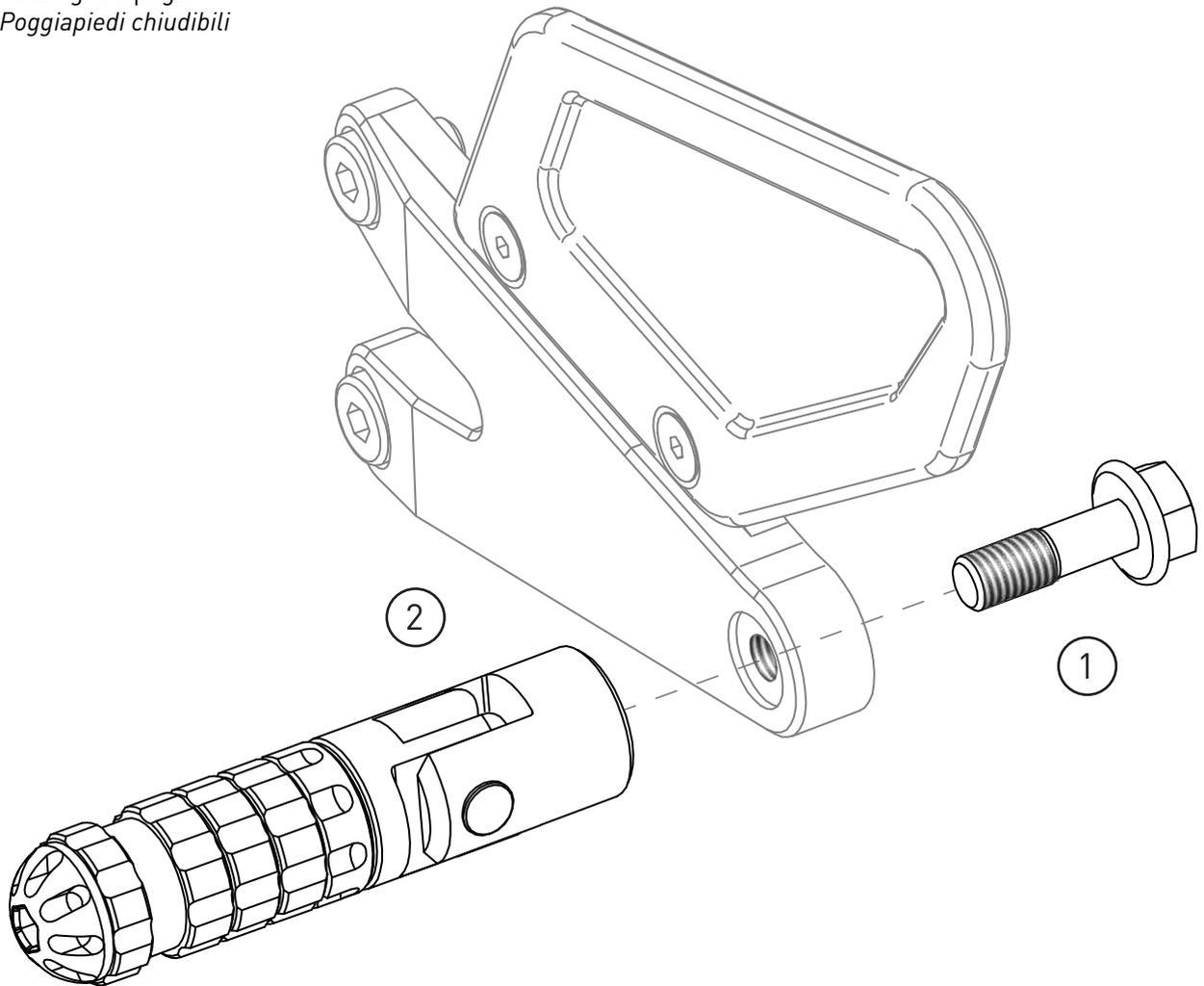
1. Screw in the special bolt completely only from the back side of the plate.
